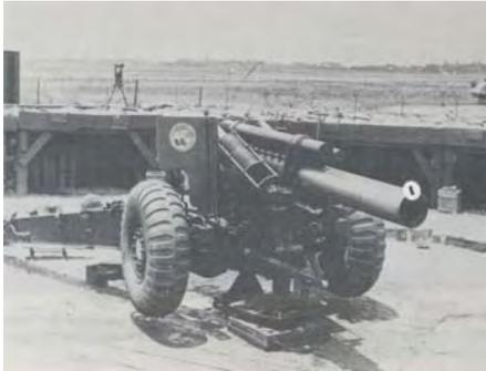
155-MM. HOWITZER POSITION USING SPEEDJACK AND COLLIMATOR.
